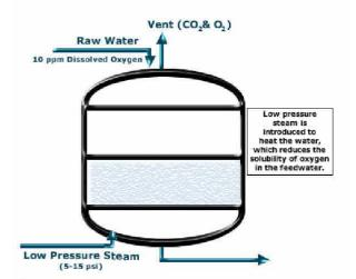
While modern mechanical deaerators can reduce the dissolv ed oxy gen level to sev en thousandths of a ppm, any malfunction of the equipment will permit much higher levels of oxy gen to enter the boiler.
