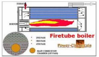
Industrial boilers are generally classified as either fire tube of water tube. This refers to the design of the boiler.
