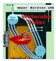
inside the tubes, while hot gases pass over and around the outside of the tubes. Water tube boilers can operate at higher press ures than fire tube boilers.
