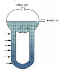
The water then flows from the drum down through the cooler rubes, or "downcomers", completing and repeating the cycle.
